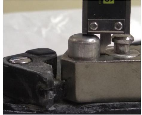
When set up, the button must overpass 6 mm only pushed by the spring.
