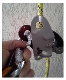
2° Close the mobile plate and fix the connector within the two holes. (fixed and mobile plates ).
