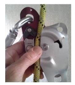
${\bf 1}^{\circ}$  open the mobile plate, connector hole of the fixed plate turned to the top, pass the rope in the middle .
